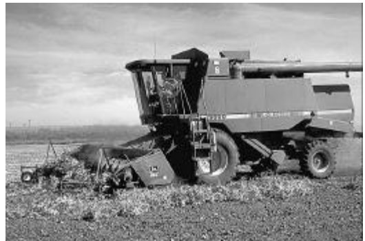
Tip 10. Harvest the bean crop when seed has reached proper moisture. Adjust combine cylinder speed, concave and other settings to prevent seed damage; monitor seed quality during harvest; air dry to 14%.
